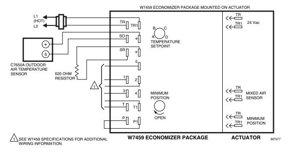
Fig. 2. Wiring Connections for C7650A Temperature Sensor.
